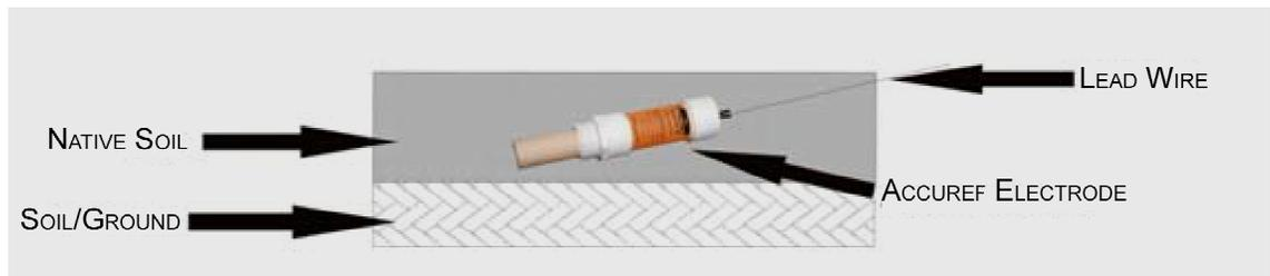
5. **NOTE:** The soil surrounding the AccuRef must remain moist and undisturbed.
